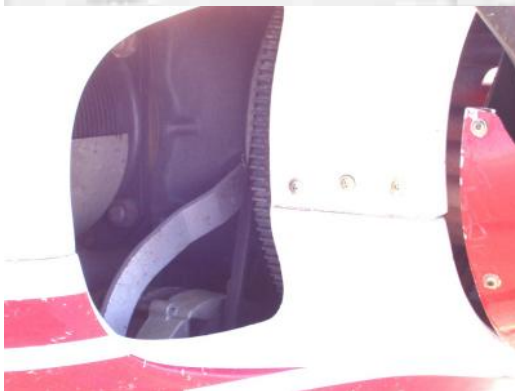
Alternator Belt – CHECK tension and condition.
