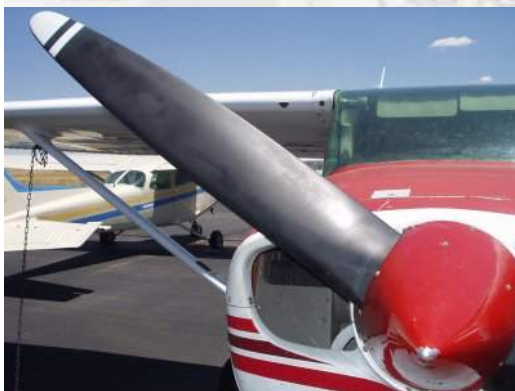
Propeller and Spinner – CHECK for nicks and security.
