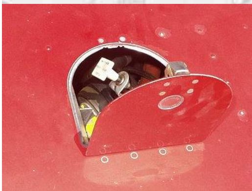
Fuel Strainer – DRAIN about 4 seconds before first flight of the day and after refueling.
